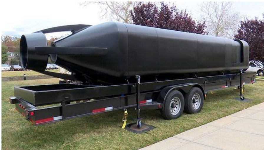
Carbon-fiber submersible produced by Oak Ridge National Laboratory using a 3-D printer.
