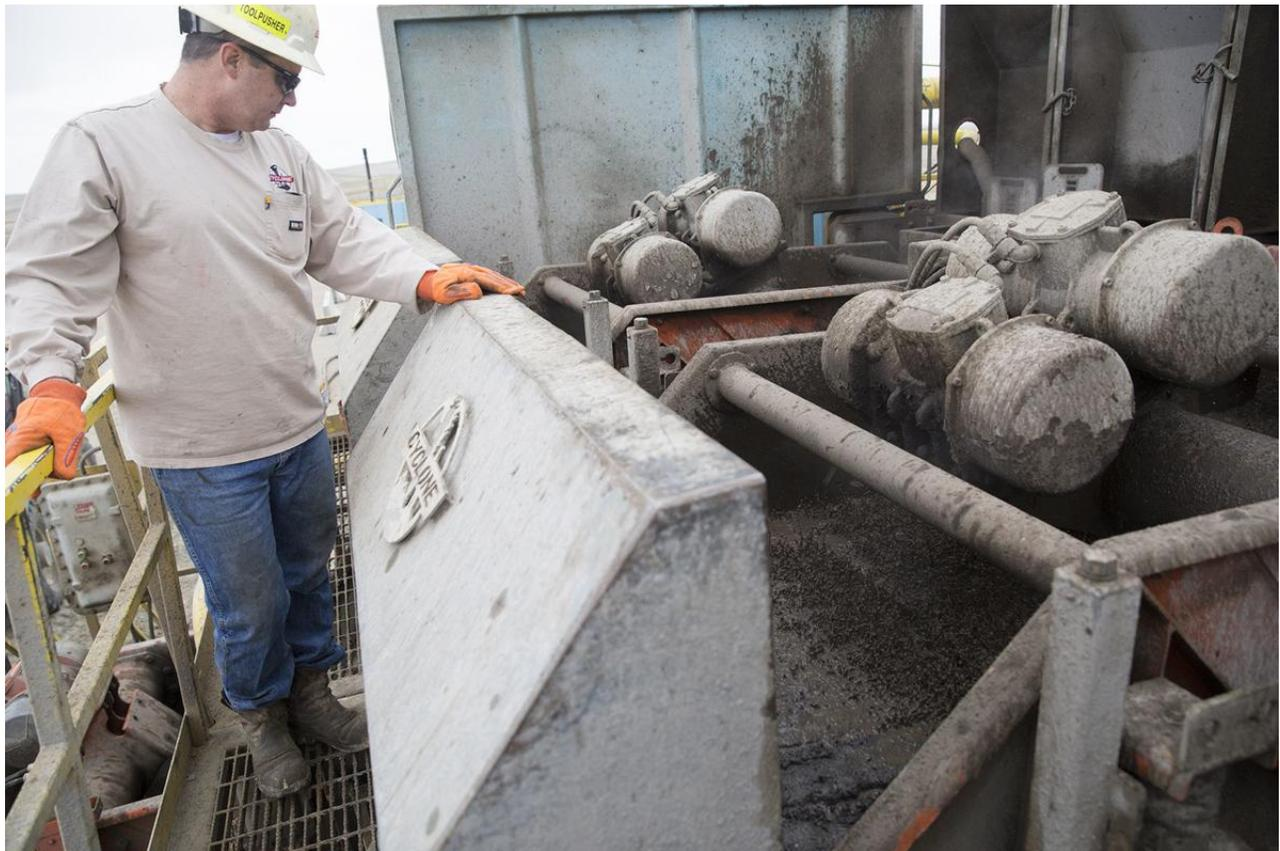
Marty Sedgwick, a rig manager for Cyclone Drilling, stands next to the shale shaker used to remove large solids from the drilling fluid Thursday afternoon on Cyclone's oil rig No. 39, working in Converse County near Douglas. News Record Photo/Kelly Wenzel
