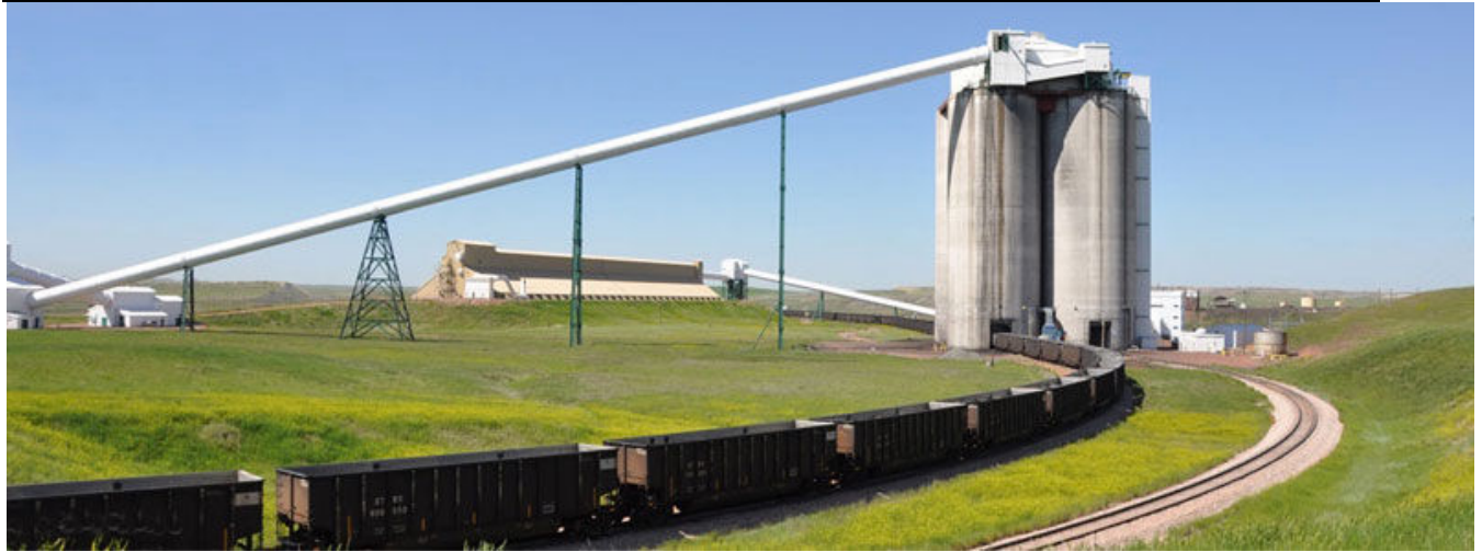
A coal train loads up at a silo at a Cloud Peak Energy mine. www.cloudpeakenergy.com
