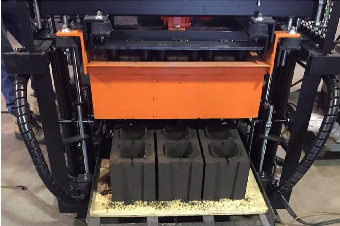
Carbocrete traps carbon in concrete blocks by using it with water in a cold curing process that replaces the traditional heat and steam. PHOTO: CARBICRETE
